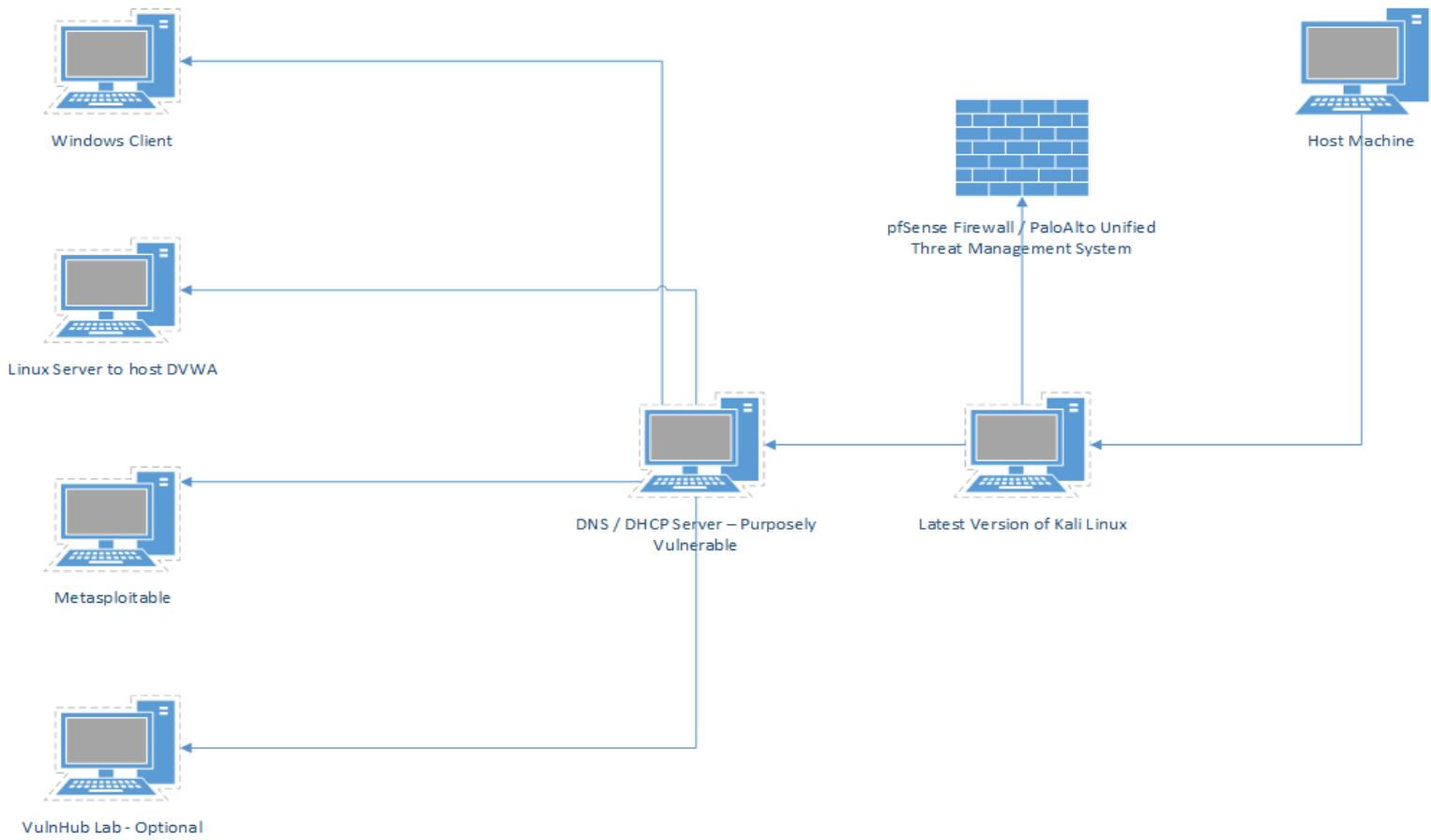
This is a logical diagram of the proposed setup. The DHCP/DNS server should be the gateway to the rest of the network hosting DNS records for any web-based application you are hosting.
