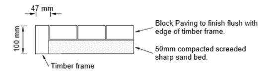
NB jointing sand to be brushed into paving on completion
