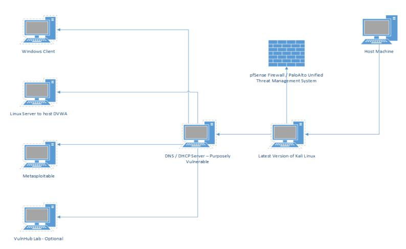
This is a logical diagram of the proposed setup. The DHCP/DNS server should be the gateway to the rest of the network hosting DNS records for any web-based application you are hosting.
