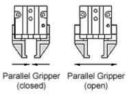
customized to suit the specific object being manipulated. The workpiece is released from the gripper when both sides simultaneously open and let go of the object.
