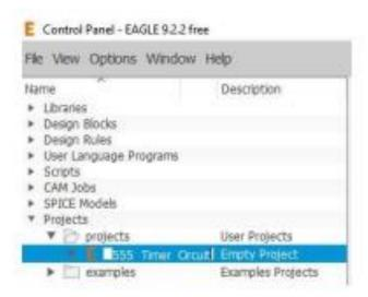
As we will be producing a schematic, we first need to add one to the project. This is done by right clicking the project name, and then 'New > Schematic.' This will add a schematic to the existing project and automatically open it.
