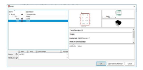
Once you have typed 'ne555?' into the search bar and hit enter, the above screen will pop up. We are going to click the drop down where it says '\*555,' and we are going to use the through hole 'DILO8' version. When you have selected it press 'OK.' We are going to left click to place the component in the centre of the schematic. Press 'Esc' to return to the 'Add Part' menu.
