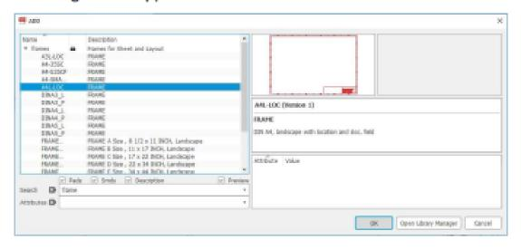
As the circuit is only small, we will only need a small schematic frame. So we will use the A4 landscape one named 'A4L-LOC.' Once you have selected it, press OK. You will notice that the bottom left hand corner of the schematic now replaces the mouse cursor. Simply left click to place the frame. Once you have done that Eagle automatically attaches another frame to the cursor in case you need to use multiples, just press 'Esc' to return to the 'Add Part' menu.
