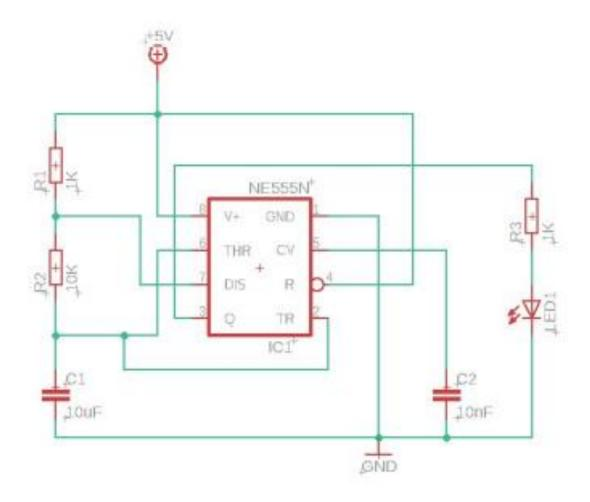
You have now produced a schematic of a functioning 555 timing circuit.
