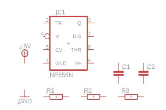
To move the components, you need to left click the red cross in the middle of each component. Alternatively, you can hold left click and drag the cursor around the group of required components. In both instances you will notice that the red outline of the component will get brighter. This means that the component is selected. You can now drag and move each component freely.
